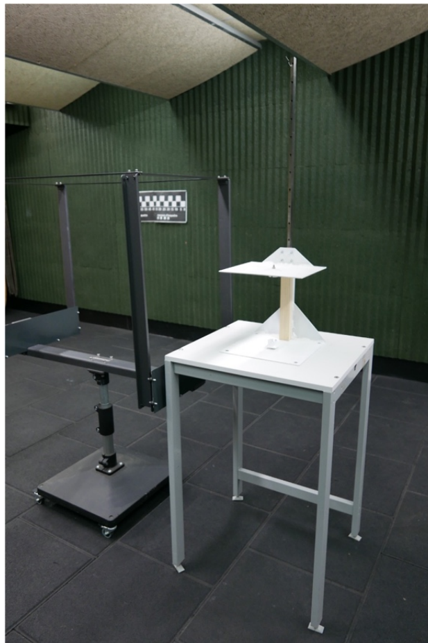
Fig. 6 Fixation table and partially depicted light barrier system in the scientific laboratory.
