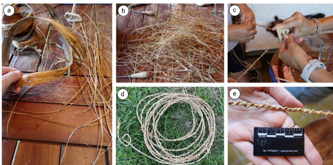
Figure 5. Experimental approach: a) wide strips of lime tree bark; b) lime tree bark after stripping; c) S z,z cord making with a rope-twisting tool ; d, e) the final rope.
