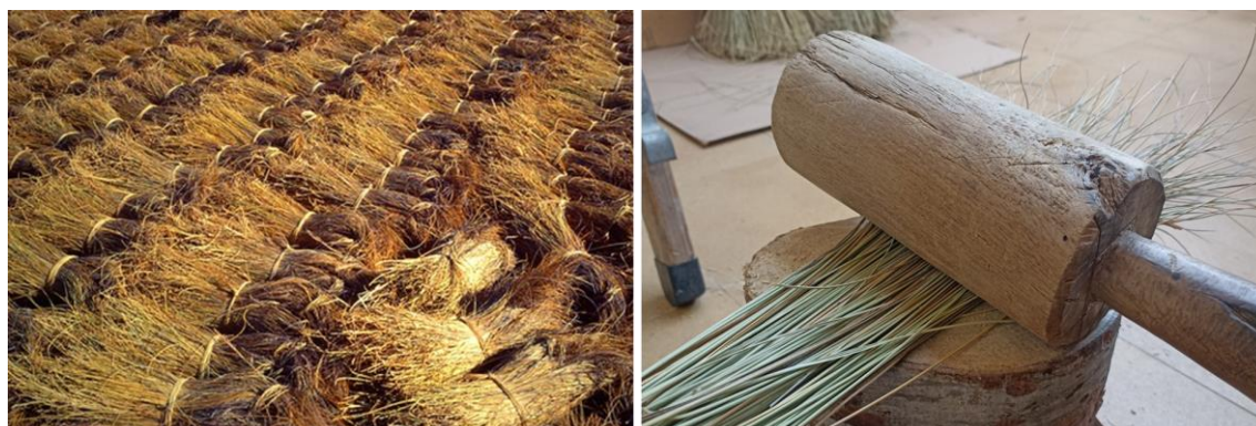
Figure 5. Left: Esparto grass being dried. Right: Traditional wooden hammer for crushing esparto leaves.
