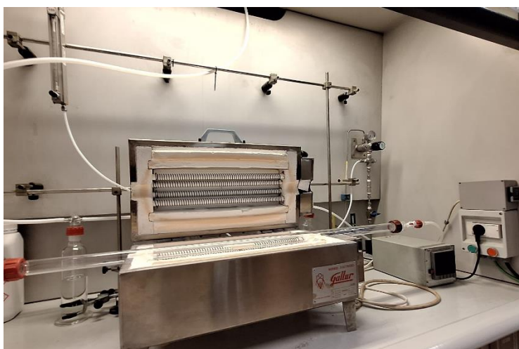
Figure 2.2. Ammonolysis furnace at the solid state chemistry laboratory of ICMAB.
