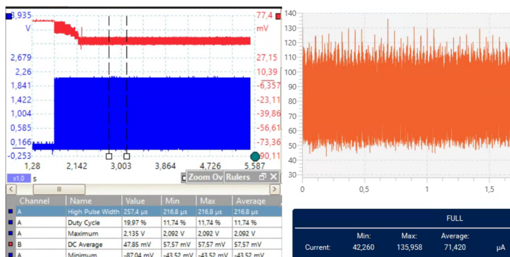
Fig. 4.60: Current consumption of the control circuit working in operating mode for V_{cc} = 2V and V_{oc} = 100mV .
