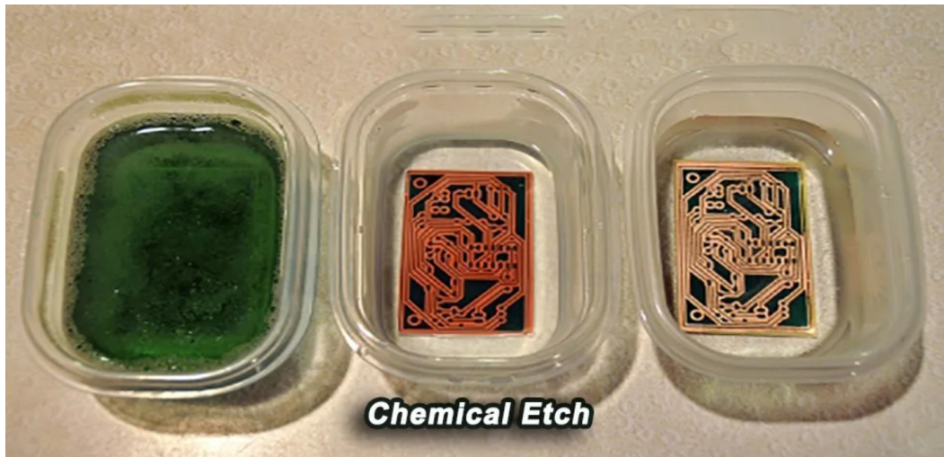
Fig. 2.5: Stages of a PCB being chemically etched to form a circuit pattern. Source: [9].
