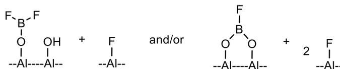
**Figure II-21.** Possible surface species for the stabilisation of  $\text{BF}_3$  using  $\text{Al}_2\text{O}_3$  as a support material.<sup>102</sup>
