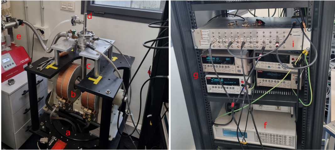
Fig. 4.3: Measurement setup. a. Motorised rotation stage. b. Electromagnet. c. Cryostat. d. Liquid nitrogen input line. e. Turbomolecular pump. f. PID temperature controller. g. Current and voltage sources and multimeters. i. Switch box.
