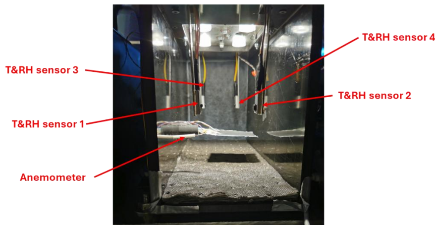
Figure 4-8 Sensor, actuators and filters placement inside the unit
