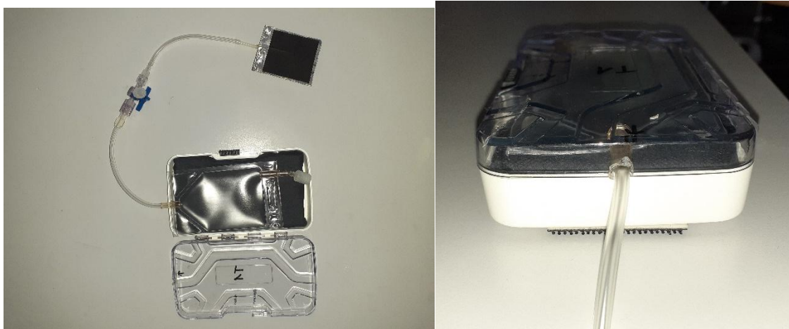
Figure 4-16 Watering tank on absorbent paper connected to the leaf replica within its enclosure (left) and outlet when closed (right).
