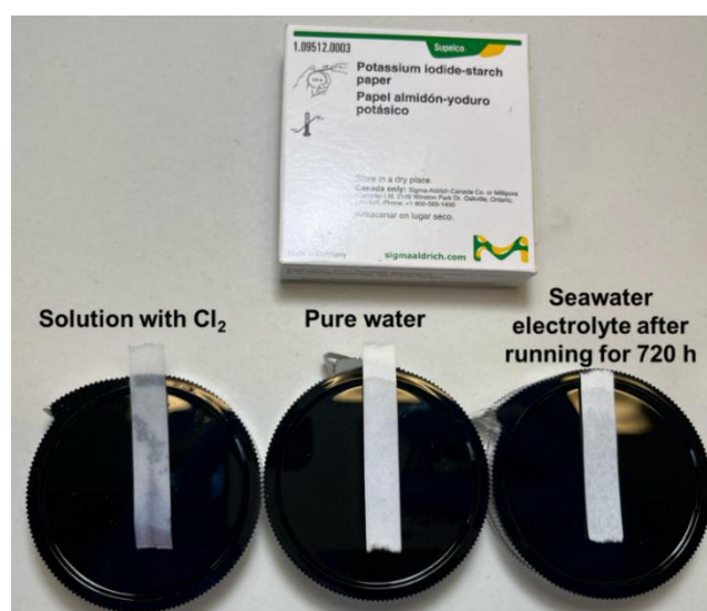
Figure 3.23 Digital photo of potassium iodide-starch paper with seawater electrolyte after running for 360 hours at the current density of 100 mA·cm -2 , and comparison with water, and solution containing Cl 2 .
