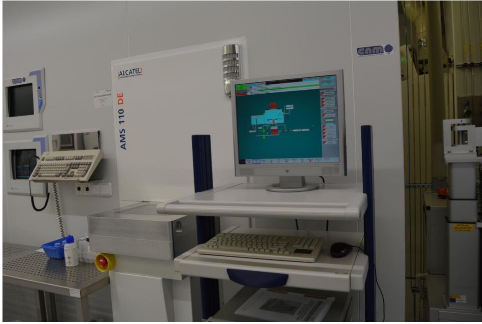
Figure 19: Alcatel AMS-110 DE dry etcher sourced from IMB-CNM-CSIC platform.
