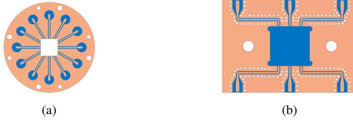
Figure 2.4: (a) Design of the PCB used to obtain the results in Ch. 3. (b) Design of the PCB used to obtain the results in Ch. 6. In both PCBs, the blue part is the ceramic substrate, while the orange part is Cu. The small holes are internally metallized with Cu, in order to electrically connect the two sides of the PCB and establish a proper grounding, whereas the big holes are for fastening screws.
