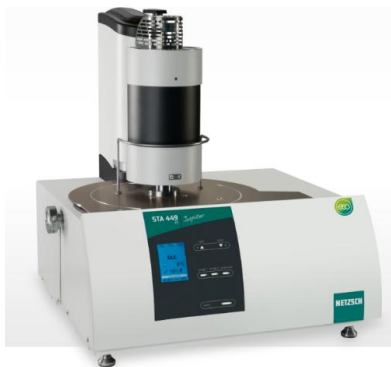
Figure II. 3. Image of the STA 449 F1 Jupiter used for TGA analysis [10].
