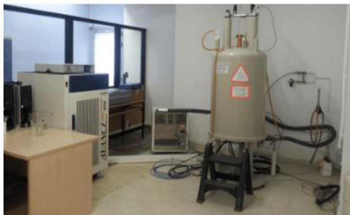
Figure II. 2. 400 MHz BRUKER nuclear magnetic resonance (NMR) spectroscopy image [8].
