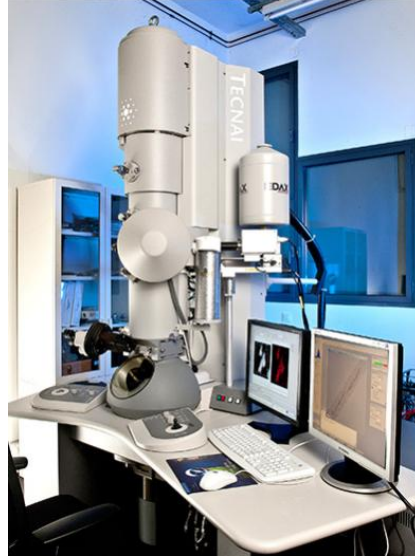
Figure II. 10. Transmittance FEI Tecnai G2 F20 electron microscope image [22].
