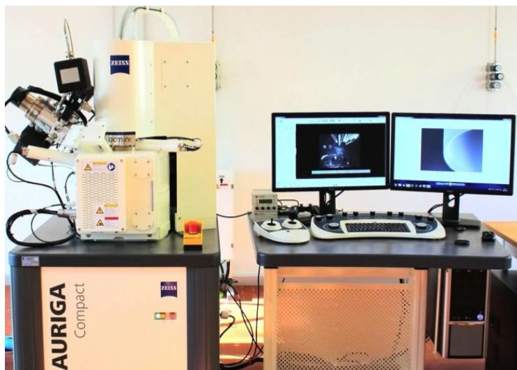
Figure II. 9. Image of an AURIGA-ZEISS scanning electron microscope equipped with an EDS spectrometer [20].
