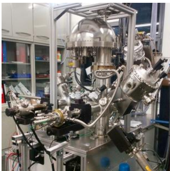
Figure II. 8. Image of the SPECS instrument equipped with a PHOIBOS 150 MCD-9 hemispheric analyzer [18].
