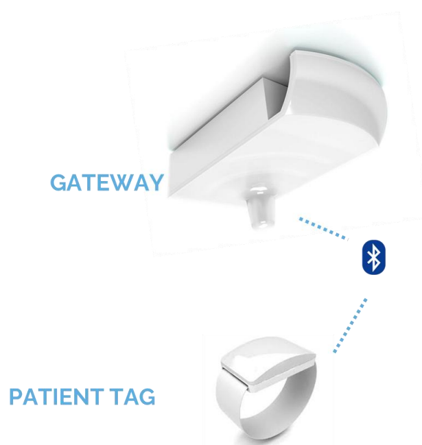
Figure 9 – Used RTLS hardware
