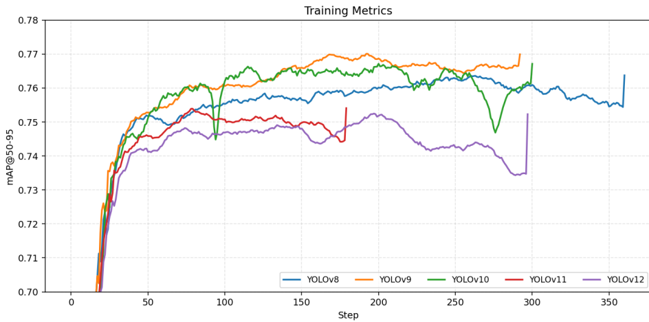
Figure 6. Training evolution of each YOLO model variant. Performance scores are based on the validation set. The last value represents the best performing epoch found before overfitting.
