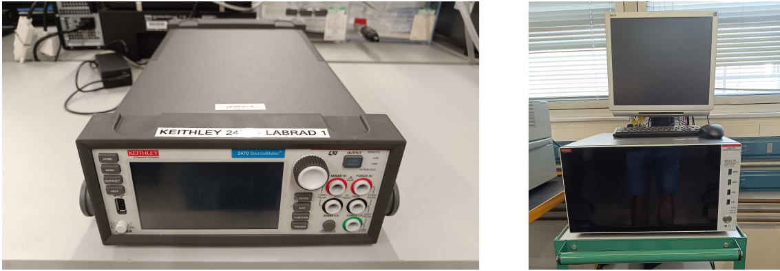
Figure 3.10: Keithley 2470 for I–V measurements on diodes (left) and Keithley 4200-SCS for additional electrical tests (right).
