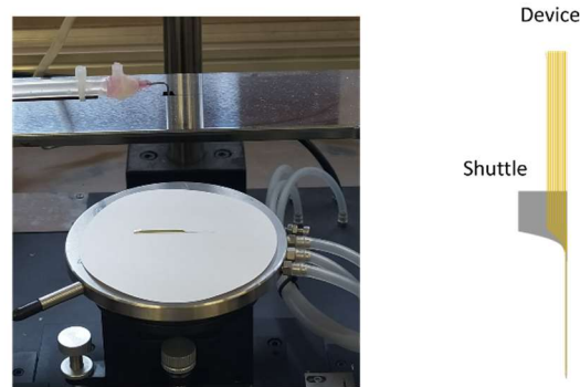
Figure 3.4 | Assembling of flexible probe onto silicon shuttle. On the left, setup used to glue the flexible device to the shuttle. The device is placed on a probe station that can be moved with manipulators. A vacuum pump connects with a plastic tube and a metallic tip that can hold the shuttle. After applying the adhesive polymer with a brush on the tip of the shuttle, the flexible device is aligned with the shuttle, looking under the microscope, and then assembled. On the right, a schematic of a device attached to the shuttle.
