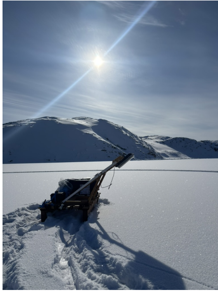
(a) ARIEL L-band radiometer deployed over snow-covered sea ice.
