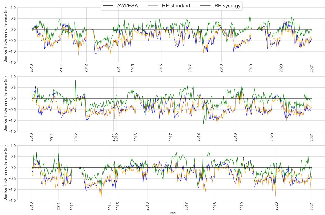
(b) Absolute thickness differences (residuals) between the satellite retrievals and the respective BGEF mooring measurements.
