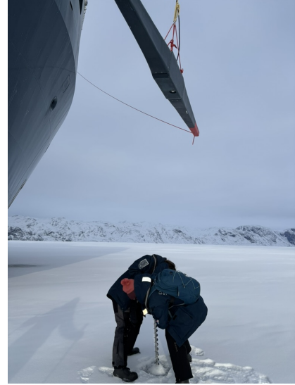
(b) Validation of the SIMS instrument, with a colocated ice drilling below during an ice station.
