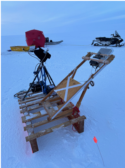
(a) ARIEL L-band radiometer deployed over snow-covered sea ice, with an infrared camera mounted on the sled.
