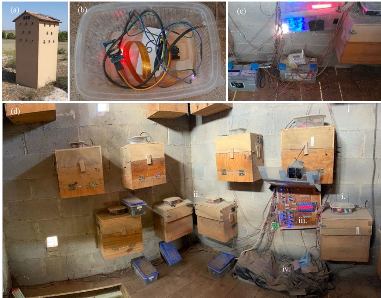
Figure 3.2 Centralised monitoring system to study reproductive behaviour in wild jackdaws. (a) Nesting tower equipped with solar panels. (b) Single child unit installed inside a dust-proof plastic box on top of a nest-box. (c) 12V batteries wired in parallel powering the system through the custom relay board controlled by the parent unit. (d) Inside view of the tower, including (i) the parent unit, (ii) child units, (iii) the custom relay board, and (iv) batteries (covered under a plastic).
