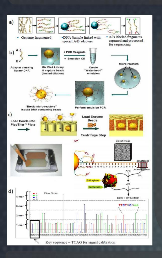
First commercialized NGS on market. It was designed by 454 Life Sciences but now belongs to Roche. This sequencer use pyrosequencing technology. When one base is added, releases Ppi, we can see a light emission thanks coupled reaction and captured with CCD camera. Fragment amplification is done using emulsion PCR. Sequencing procedure is realized in plate with 1,6 millions of wells. Every well only can support one bead.
