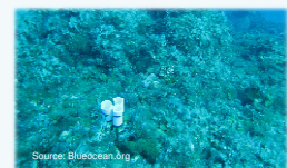
Image 7. Sediment trap in situ.
