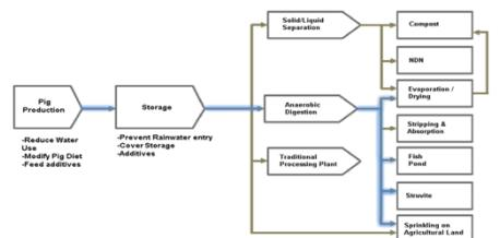
FIGURE 2: ALL PROCESS ALTERNATIVES. PROCESSES HIGHLIGHTED IN BLUE HAVE HAD THEIR ENVIRONMENTAL EFFECTS ANALYZED TO SEE WHICH ONE WOULD BE MOST PROMISING TO IMPLEMENT AS FURTHER ADDITIONS TO THE ANAEROBIC DIGESTION.
