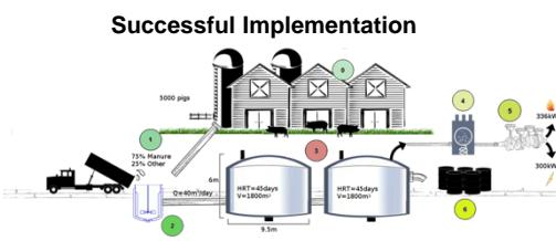
FIGURE 4: CONCEPTUAL REPRESENTATION A BIOGAS DIGESTION PROCESS OBSERVED IN CASSÀ DE SELVA, GIRONA. MAIN DIFFERENCES WITH THE PROPOSED PROCESS ARE:
