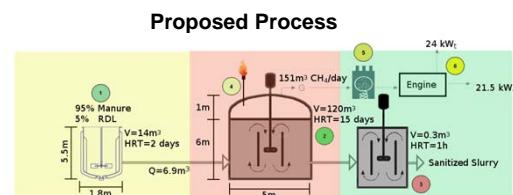
FIGURE 3: SCHEMATIC REPRESENTATION OF THE CHOSEN PROCESS DESIGN. IT CONSISTS OF:
