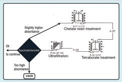
After the stream undergoes the ultracentrifugation step it is expected to have an albumin coloring inferior to 0.015 absorbance units, calculated as an average absorbance at 350nm and 280nm. At the point where a sample is sent to spectrophotometer, in the case that the coloring parameter is higher to 0.015 units, measures have to be taken:
