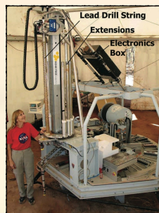
Figure 3: A photograph of the M.A.R.T.E. drill mounted on the lander.
