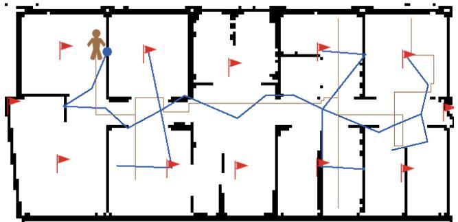
Fig. 5. Localization by centroids. The thin brown line is the real path. Blue and thicker line is the simulated path, resulting of the union of the detected positions.
