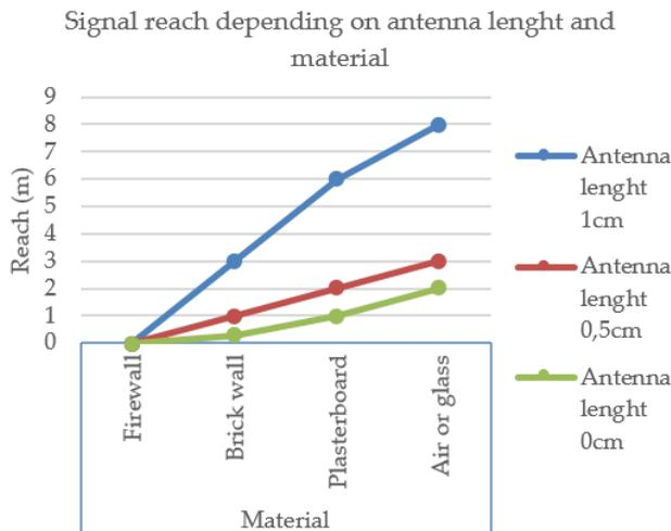
Fig. 6. Signal reach analysis. The ideal signal reach would be stronger on the brick and plasterboard walls in order to have a similar coverage.
