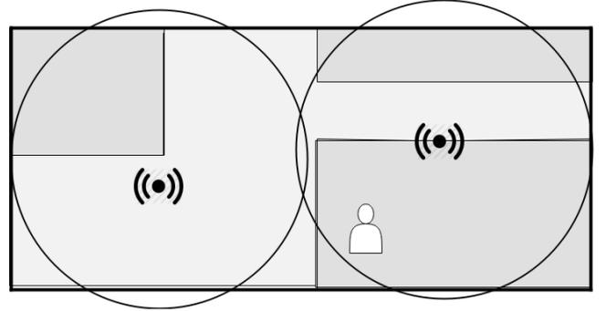
Fig. 1. Position calculation based on the nearest receiver. A floor plan with three rooms, two receiver and a person can be observed.
