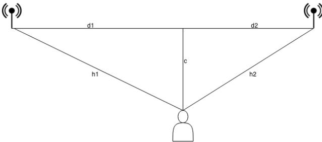
Fig. 2. Position calculation based on the time of flight
