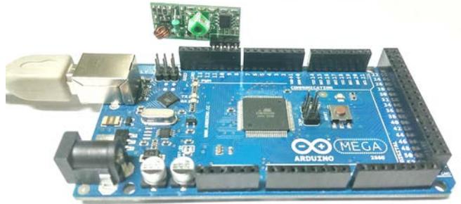
Fig. 7. Arduino Mega 2560 attached with a 433MHz receiver acting as the fixed receiver element.
