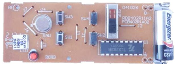
Fig. 8. 433MHz remote control acting as sender and located
