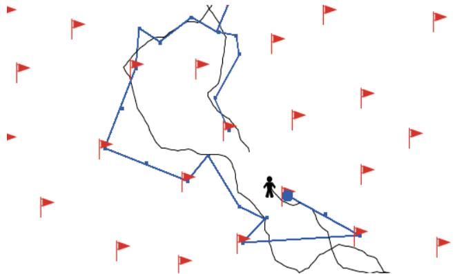
Fig. 3. Simulation of a center of masses localization system. The flags are the receivers, the black line is a random path that simulates someone walking randomly across the plane, and the thicker blue line is the estimated path.
