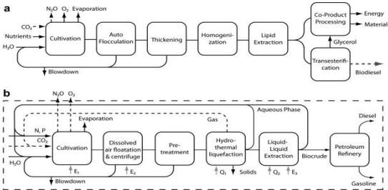
Figure 4: Flow chart of the biofuel production process. A) Old production process, producing biodiesel by transesterification. B) New production process, producing diesel and gasoline by HTL. Source [7]
