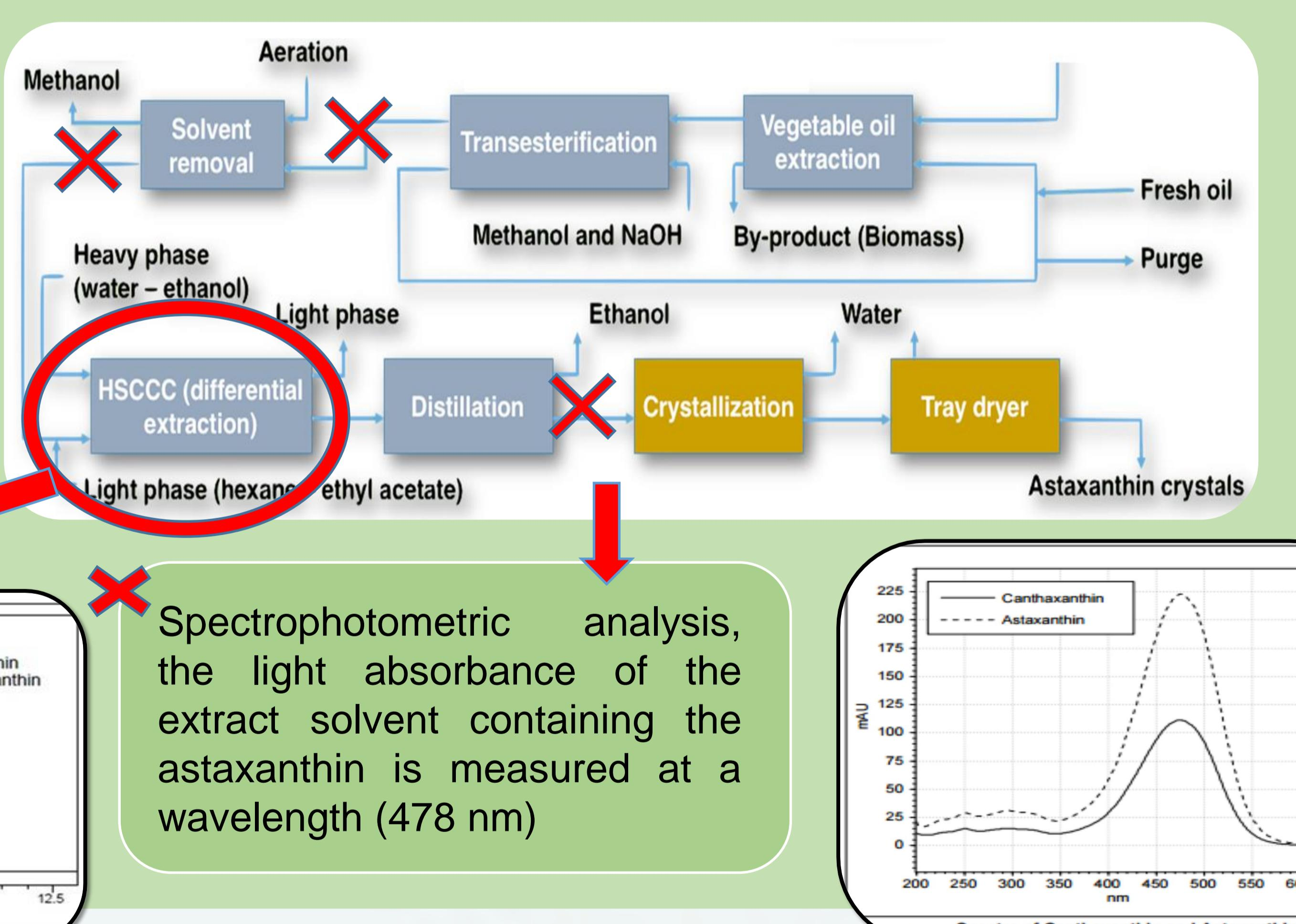
Spectrophotometric analysis, the light absorbance of the extract solvent containing the astaxanthin is measured at a wavelength (478 nm)
