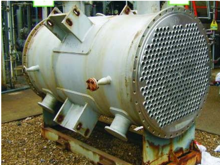
Figura 2.6 Exemple reactor carcassa i tubs industrial.
