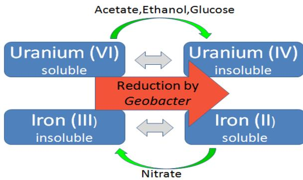
Fig. 1 Uranium and iron cycle
