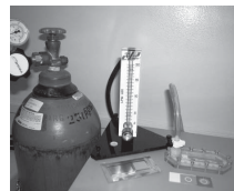
Figure 6. Evaporative drying system for sperm. Compressed ultrapure nitrogen gas is blown through a regulator and flow meter into the drying chamber, and out through a hole at the right end of the drying chamber.
