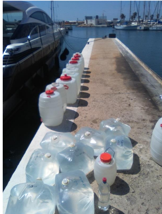
Figure 31: Plastic carboys with seawater samples filtering in Aiguadolç harbour.
