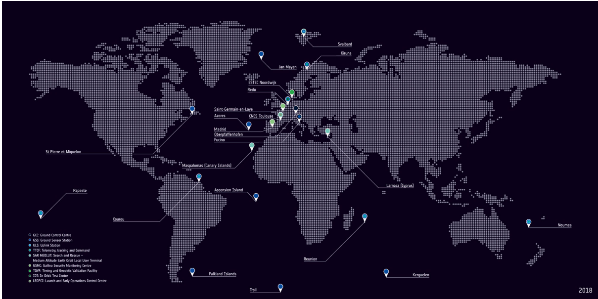
Figure 2.3: Galileo’s control segment stations around the world.
