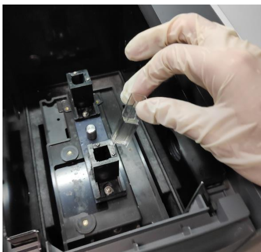
Figure 5. A UV-Vis spectrophotometer (Shimadzu UV-2600) was used to measure the OD600 of KX culture.
