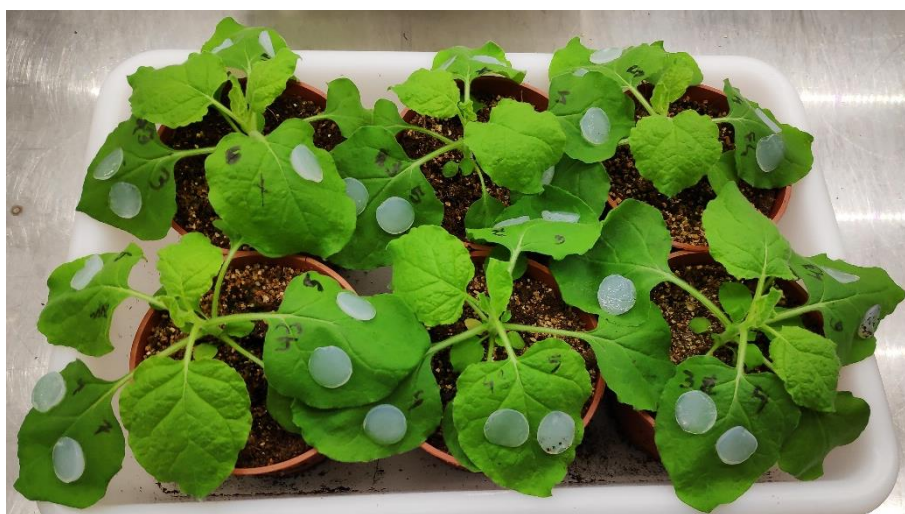
Figure 3. BC membranes covering wounds on a N. benthamiana leaf during a quality test.
