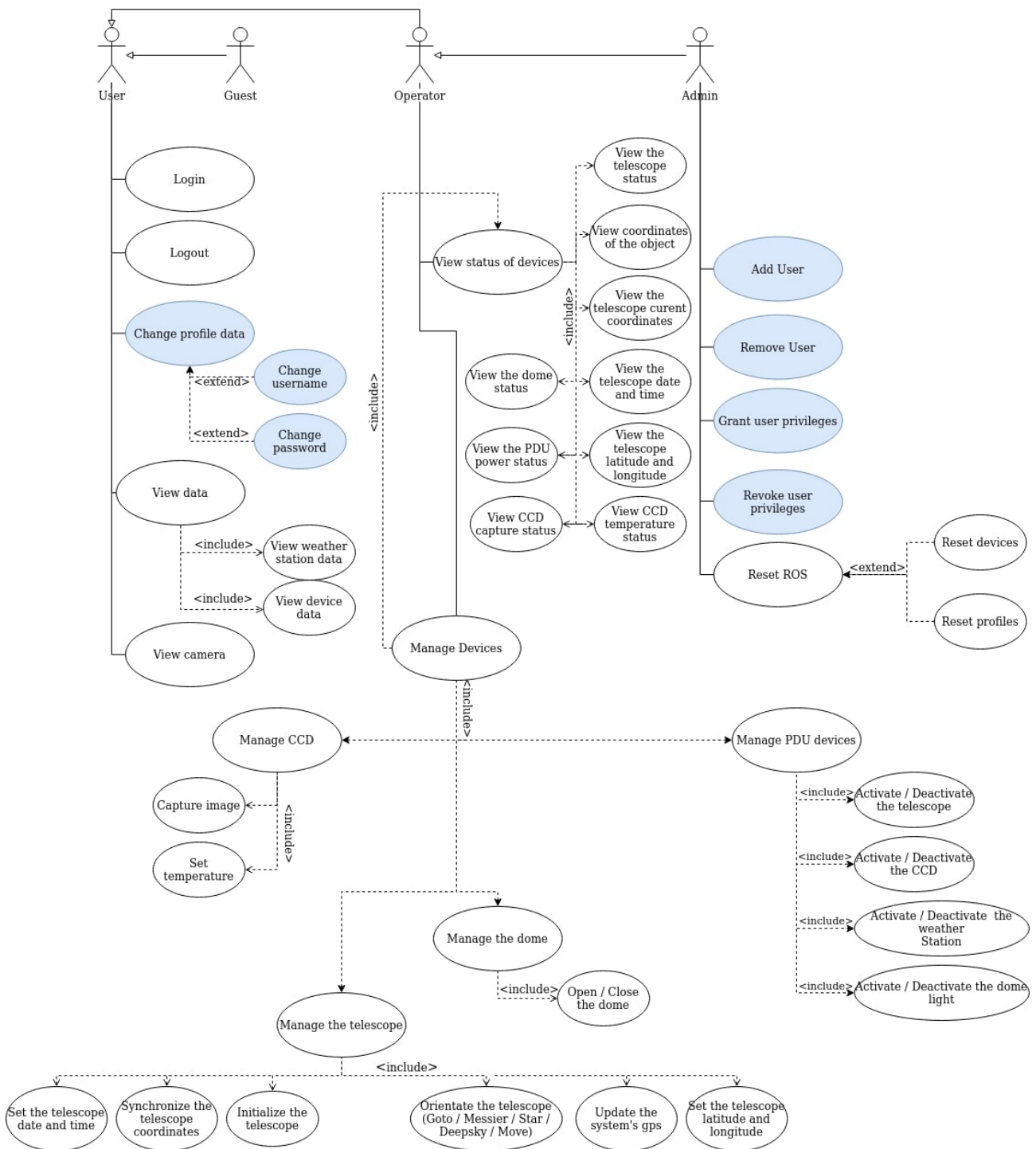
Fig. 33: Complete use case diagram. The blue colored use cases are not considered in the current SRS document.
