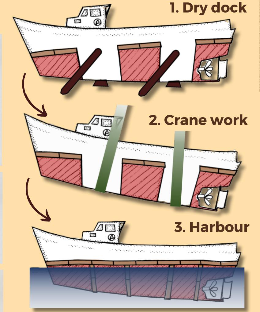
Plastic coating (red) & wood slats (light brown) are placed in the bow, stern and the hull central area, leaving sections with support structures (dark brown) free.
