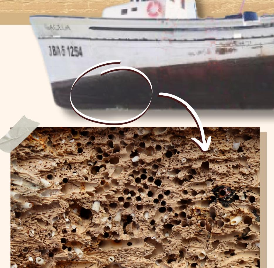
60% of hull reparations are associated with Marine Wood Borer damage
