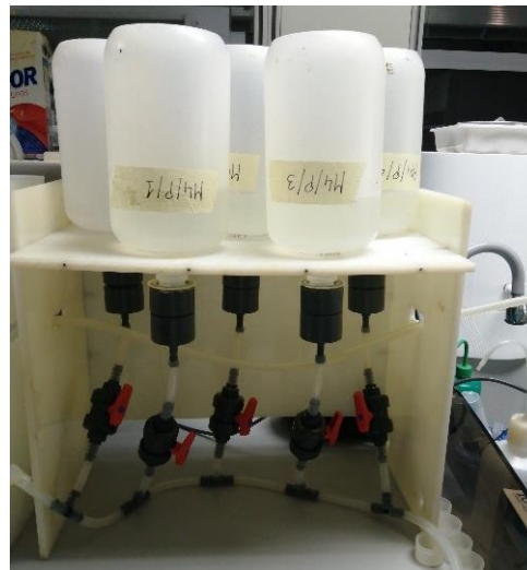
Figure 5. Picture of five samples being filtered onto the QMA filters at UPCT.
