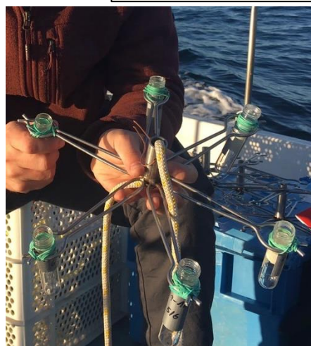
Figure 7. Picture of the metal clamps with the 6 test tubes attached with plastic rubber bands.
