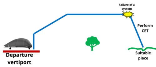
Figure 3.13 Flight path for the Basic category. From [61] and modified with Canva
