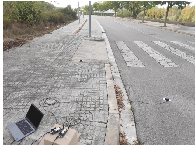
Fig. 11: Outdoor tests with two ArduSimple modules using an ICGC geodesic reference point.
