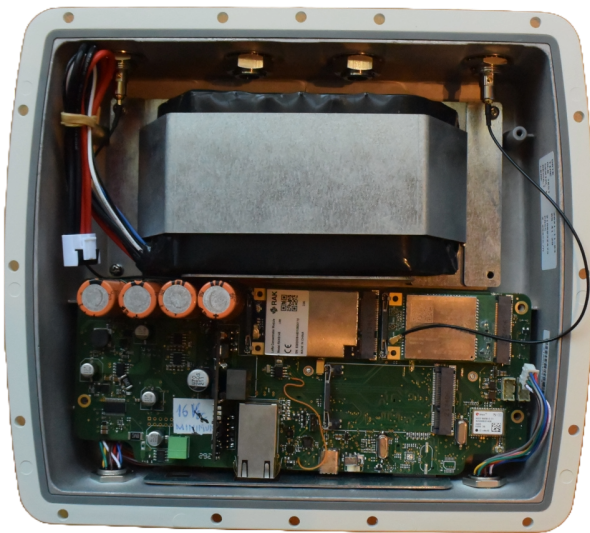
Fig. 9: Triumph node with all the equipment to be placed outdoors, including a battery and protection box.
