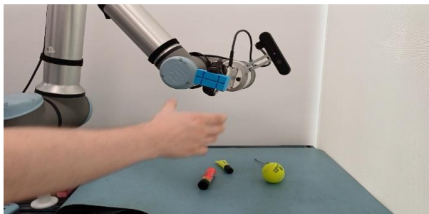
Figure 15: Robot giving the object to the user.
