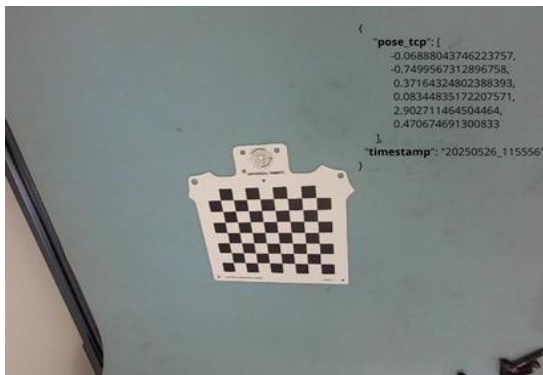
Figure 6: Example of calibration image. Can also see the exact pose of the TCP when it was taking.
