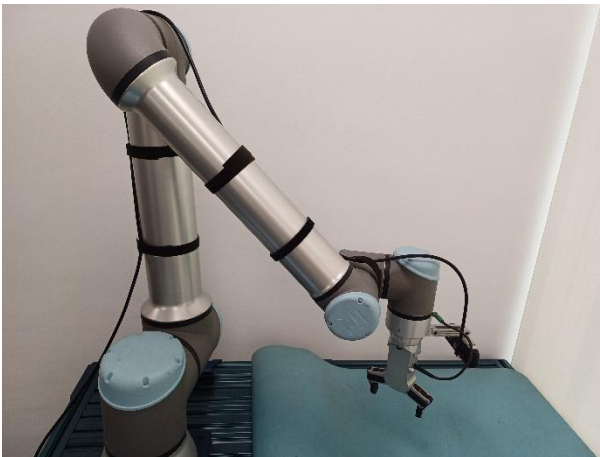
Figure 3: Robot with camera and gripper mounted
