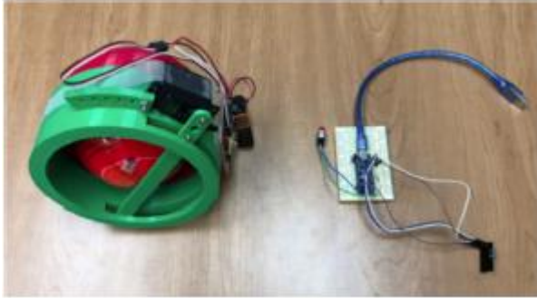
Figure 3.6 Prototype of a ball-release mechanism (left) and remote starter circuit (right), both attached to the UAV. Source: [12]
