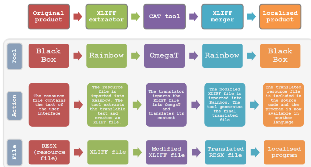
Figure 6. Simple localisation workflow using XLIFF
