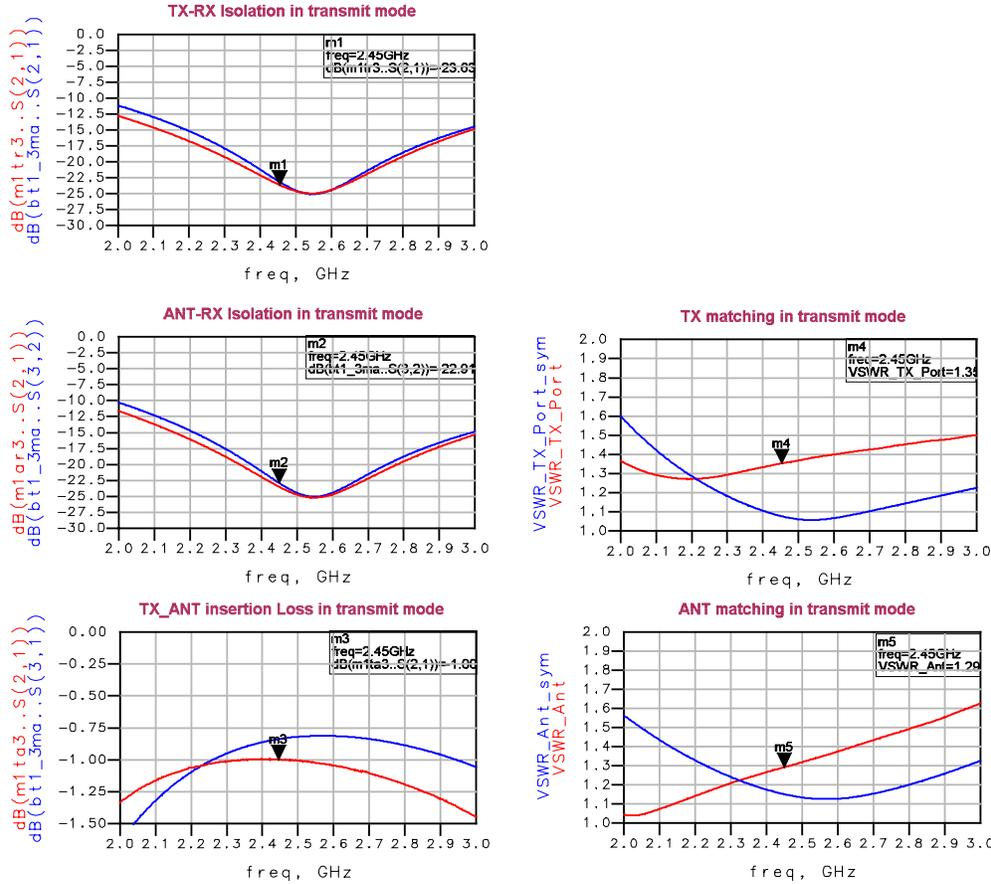
Figure 9; Results in TX mode; red curves are measurements, blue curves are the simulated ones.
