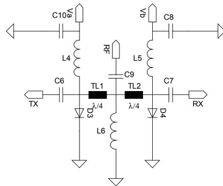
Figure 2. SPDT switch with  $\lambda/4$  sections to permit shunt diodes
