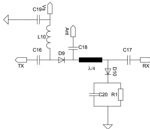
**Figure 4.** SPDT switch with a combination of a series and a shunt connected PIN diode.
