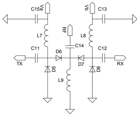
**Figure 3.** SPDT switch with series shunt diodes which results in high isolation
