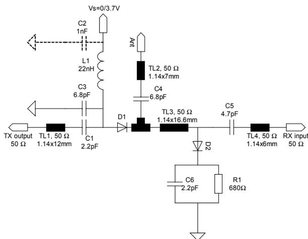
Figure 7; circuit diagram
