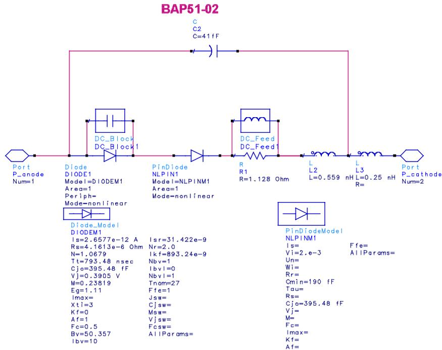
Figure 6; BAP51-02 Small Signal Model for an ADS environment
