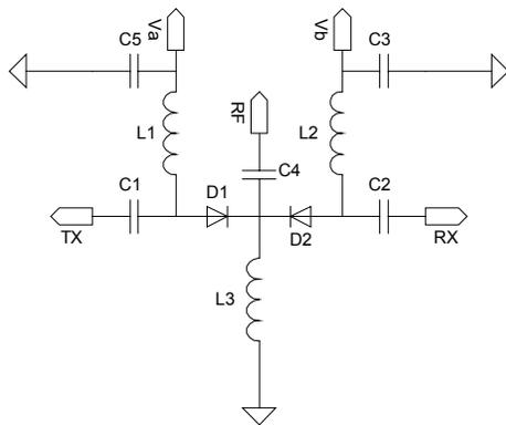
Figure 1. SPDT switch with series diodes
