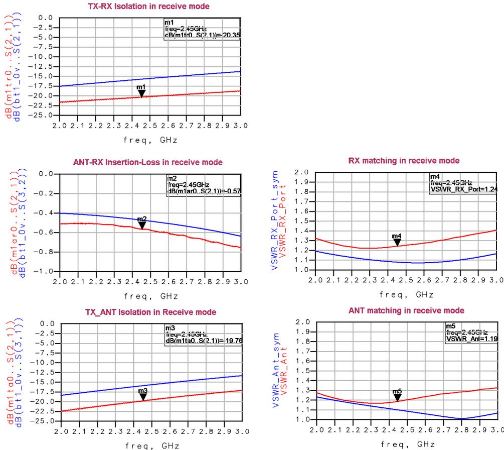
Figure 10; Results in RX mode; red curves are measurements, blue curves are the simulated ones
