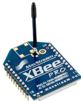
Figura 11. Transceiver XBee-PRO ZNet 2.5 RF Module
