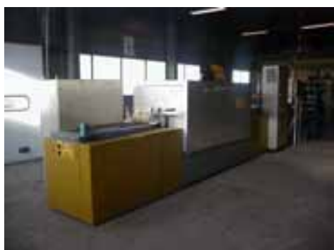
Image 1: Pilot line of continuous annealing in St-Chely
