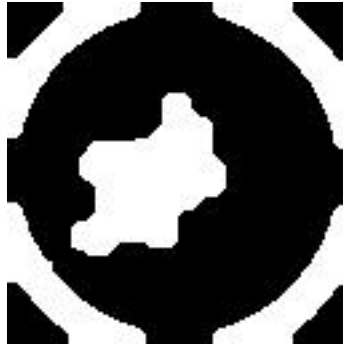
Figure 3.6 – Morphological closing on the image from figure 3.5 (parameters: disc element, radius of 6 pixels).
