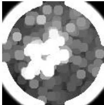
Figure 3.5 – Morphological dilation on the image from figure 3.4 (parameters: disc element, radius of 6 pixels).
