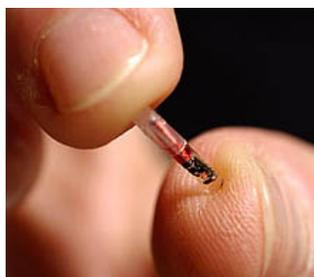
**Figura 3.16 Chip implantable de VeriChip [26]**
