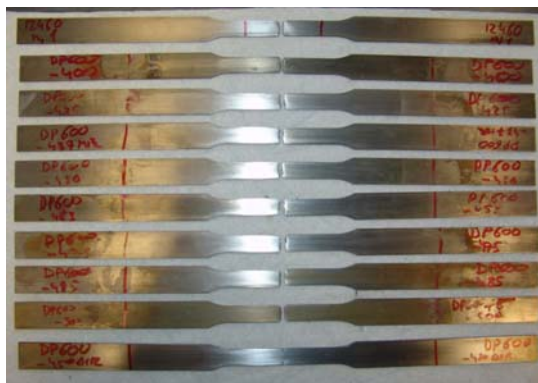
Fig 40: DP600 broken samples
