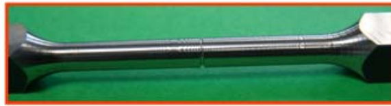
Fig 34:: The orange lines delimit the surface in contact with the electrolyte.
