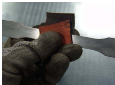
Fig. 28: Grinding a sample
