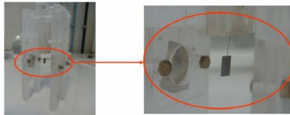
Fig. 22: Detail of the sample between the two platinum disks
