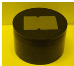
Fig 43a: DP980 sample embedded on a resin matrix
