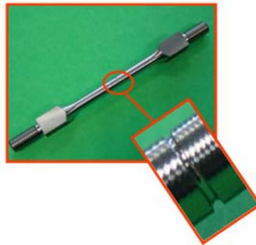
Fig. 32: Notch detail of a S700MC round sample
