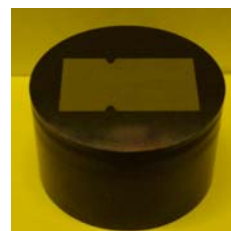
Fig 43b: S700MC sample embedded on a resin matrix
