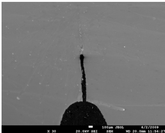
Fig. 54: crack on the left notch of S700MC sample
