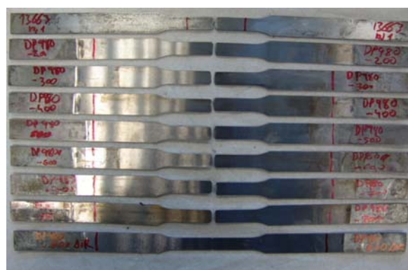
Fig. 42: DP1200 broken samples (wrong written)
