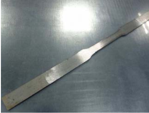
Fig 35: DP1200 sample with Zn coating removed.
