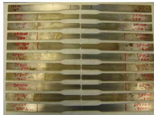
Fig 41: DP980 broken samples (wrong written)
