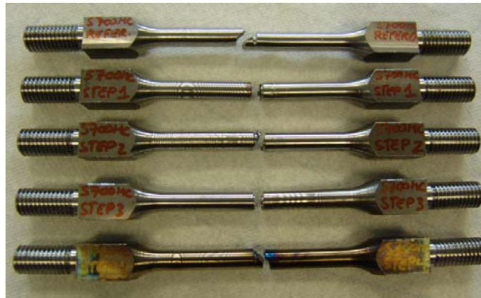
Fig. 29: S700MC notched round broken samples for incremental steps loading
