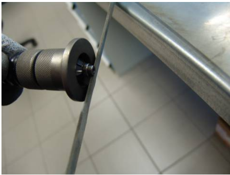
Fig. 27a: Rounding a sample's edges
