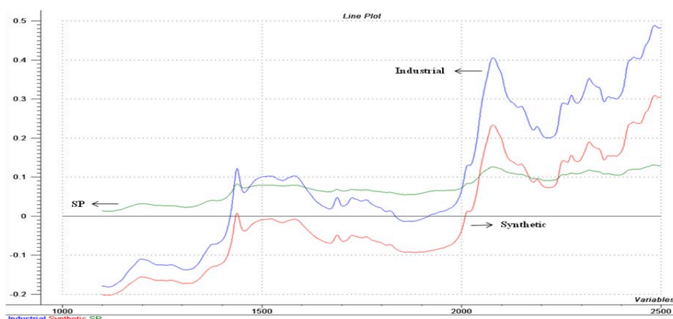
Fig 12. Absorbance spectra for a powder laboratory sample, a granulated industrial sample and a process spectrum
