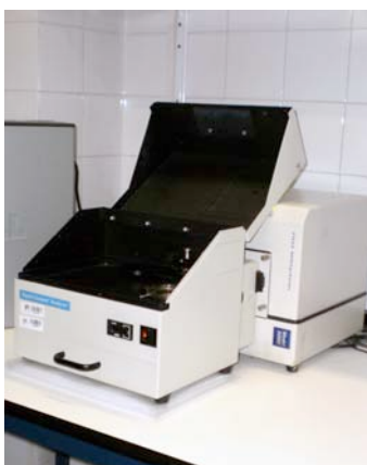
Fig7. Near Infrared spectrophotometer coupled to a RCA module
