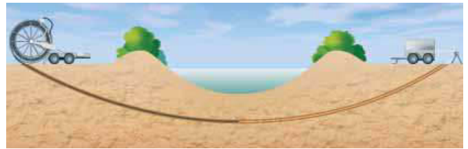
Fig. 27 Horizontal directional drilling technique
