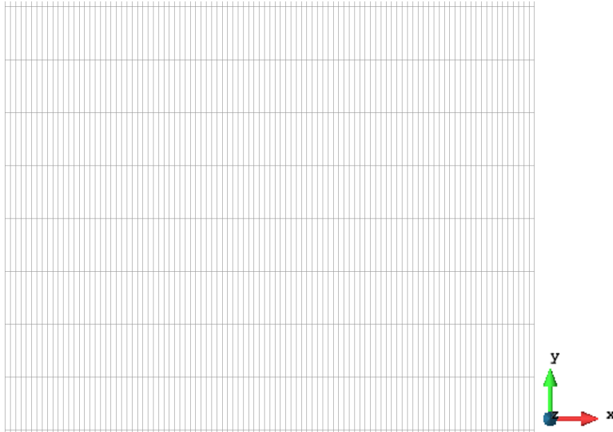
Figure 6.2.1: Detail of the mesh used in the two-dimensional slab case (10201 nodes and 10000 elements).
