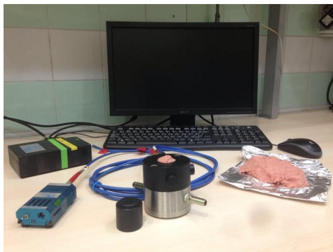
Figure 1. Optical device used to obtain the optical data from the meat emulsions.
