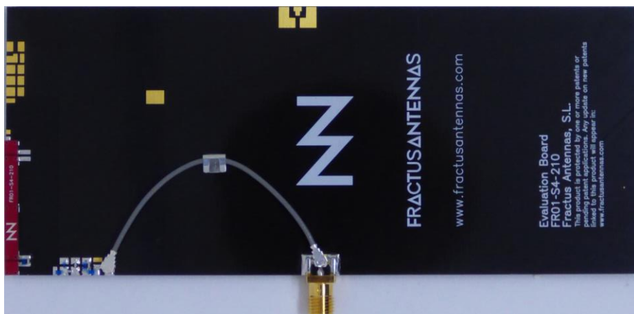
Figure 17 – 130mm x 60mm ground plane final solution.
